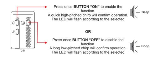
In both cases, the system will move on to the next function. Repeat the above steps to enable or disable other functions. When the last function is programmed, in addition to the confirmation tone, to indicate the end of the programming procedure, the system gives 2 low-pitched chirps, 1 high-pitched chirp and the turn indicators flash twice.
