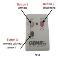
The 938 dash-mount remote control can be used to arm the whole system or arm the system partially excluding the volumetric sensors. This last option is useful when people are onboard because it does not alter the perimeter protection.
