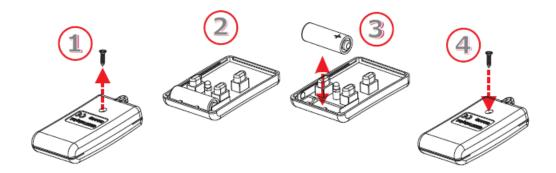
**ATTENTION:** Use only 23AE batteries. Different type batteries can seriously damage the remote control. Discard used batteries properly in special dedicated containers.
