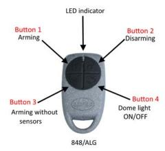
The 848/ALG remote control has a low battery charge indicator that gives you early warning to avoid malfunctioning. When the batteries are fully charged, the indicator LED will show a steady light at the press of a button. If the batteries are low, the LED will start blinking rapidly when the button is pressed.
