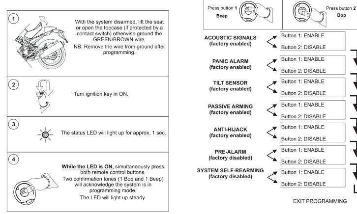
After pressing both buttons simultaneously (step 4), program the features according to your needs.
