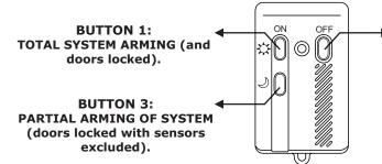
BUTTON 2: SYSTEM DISARMING (and doors unlocked).
