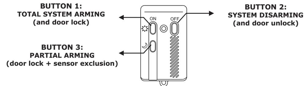
If the LED blinks 3 times at the press of a button, the battery is weak and must be replaced as follows:
