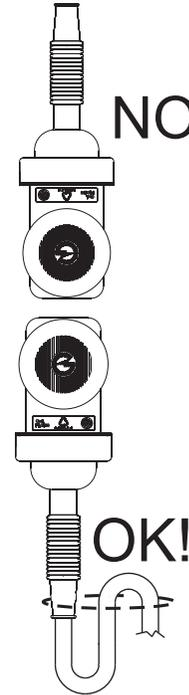
Do not install the alarm unit in this position as water ingress over time may seep through the rubber sheath and permanently damage the electronic circuit making the alarm unreliable.
