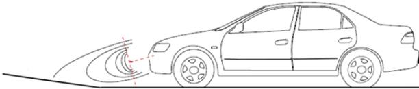
Sensors are excessively turned downwards => false alarms due to ground detection.
