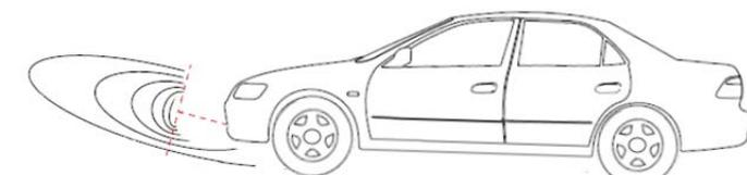
Sensors have been properly fitted but the vehicle weight has changed => the performance of the parking system is affected by the added weight.
