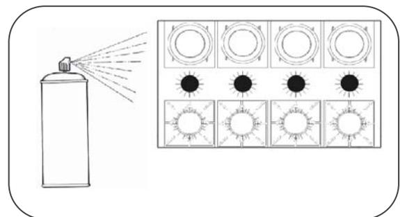
4. Fold the cardboard template into a box. Spray paint the sensors and the adapters and let dry thoroughly before assembling.
