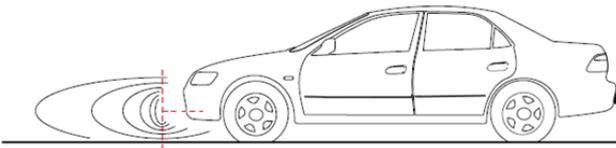
Sensors fitted too low => false alarms due to ground detection.
