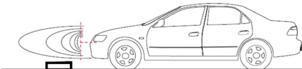
Sensors fitted too high => low obstacles are not detected.
