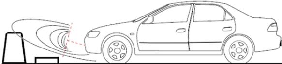
Sensors are excessively turned upwards
