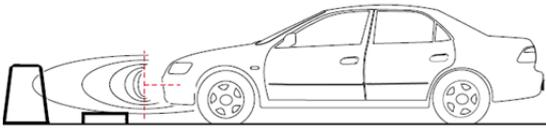
Correct Position: height, inclination and orientation are correct.\*
